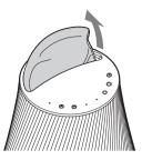
2 Remove the 2 screws using a screw driver, then lift up the top panel of the unit.
